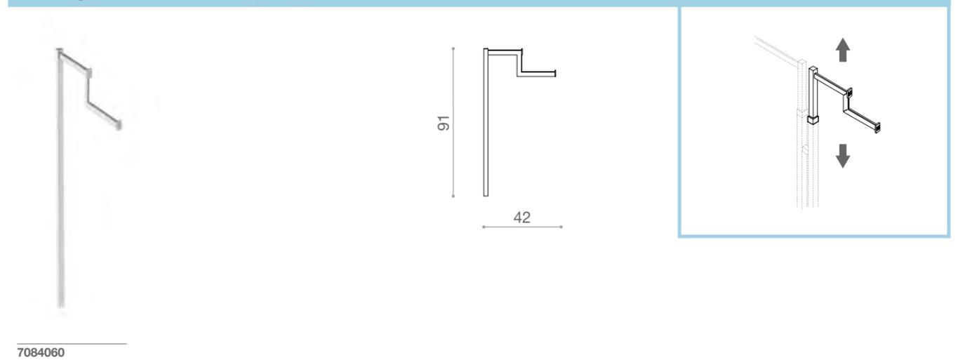
Diagram showing a 2-level hook adjustable pole. Dimensions: 91 (height), 42 (width).
